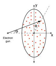
Direction of the gun can be defined using  $\theta$  and  $\phi$ . We want to hit the sheet with a uniform distribution, i.e. electron marks (red dots) on the sheet are uniformly distributed.
